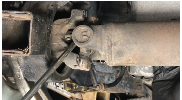
Remove half shaft, 80-82's will require a little help from a prybar
