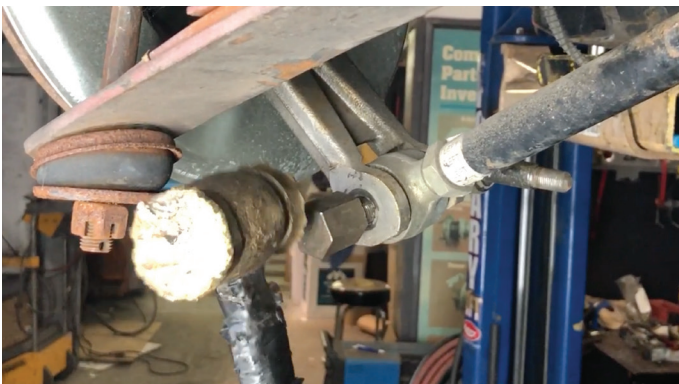
Use the castle nut or our SM-01 removal tool to knock the shock mount out.
