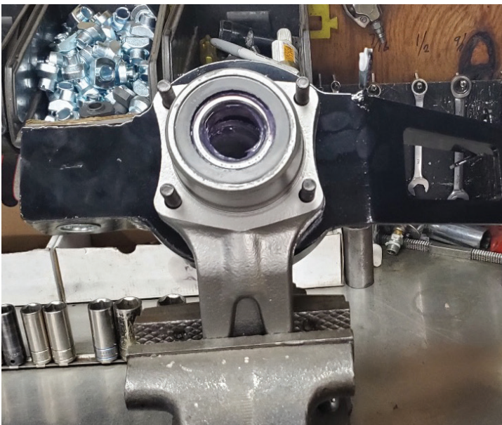
How the t-arm studs slide onto a bare bearing support.
